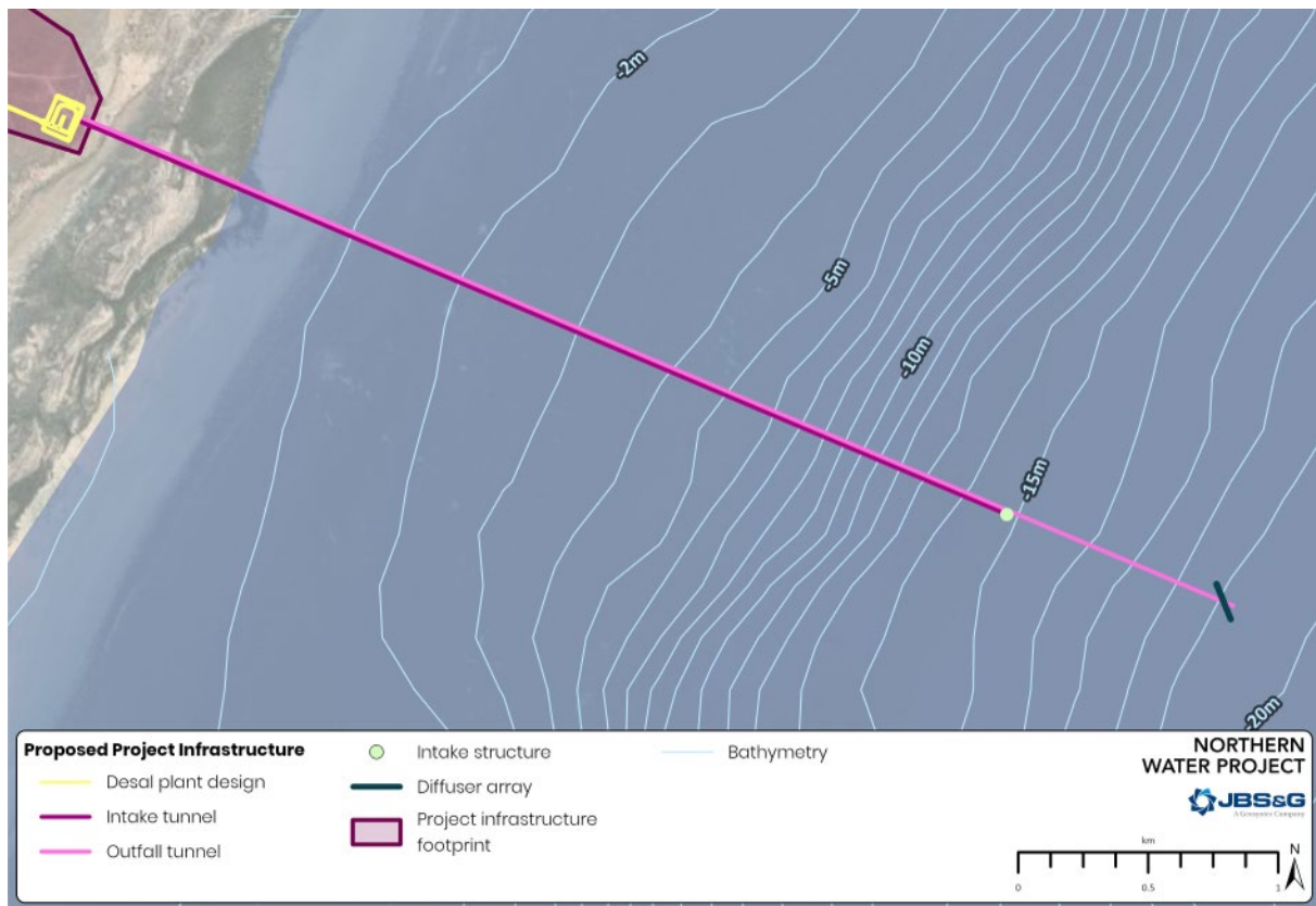
Proposed intake and outfall alignment (Bathymetry is in mAHD)
