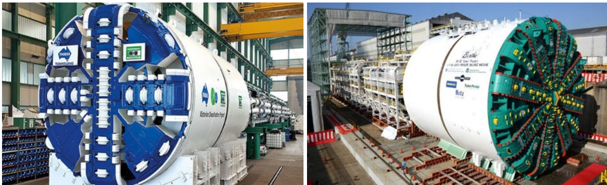
Example of slurry TBM (left) and earth pressure balance TBM (right)
